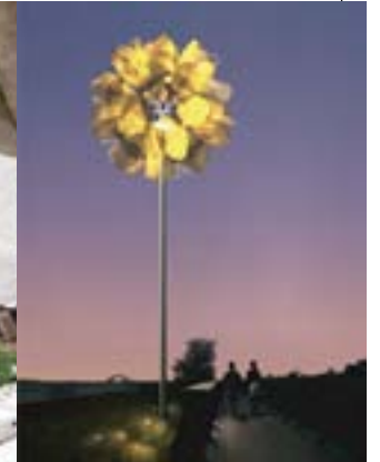
Wind-Powered LED Flower Light, Halton, United Kingdom. As wind blows at speeds above 5 miles an hour, three wind turbines attached to the flower's stem collect energy and power LEDs beneath the petals.
