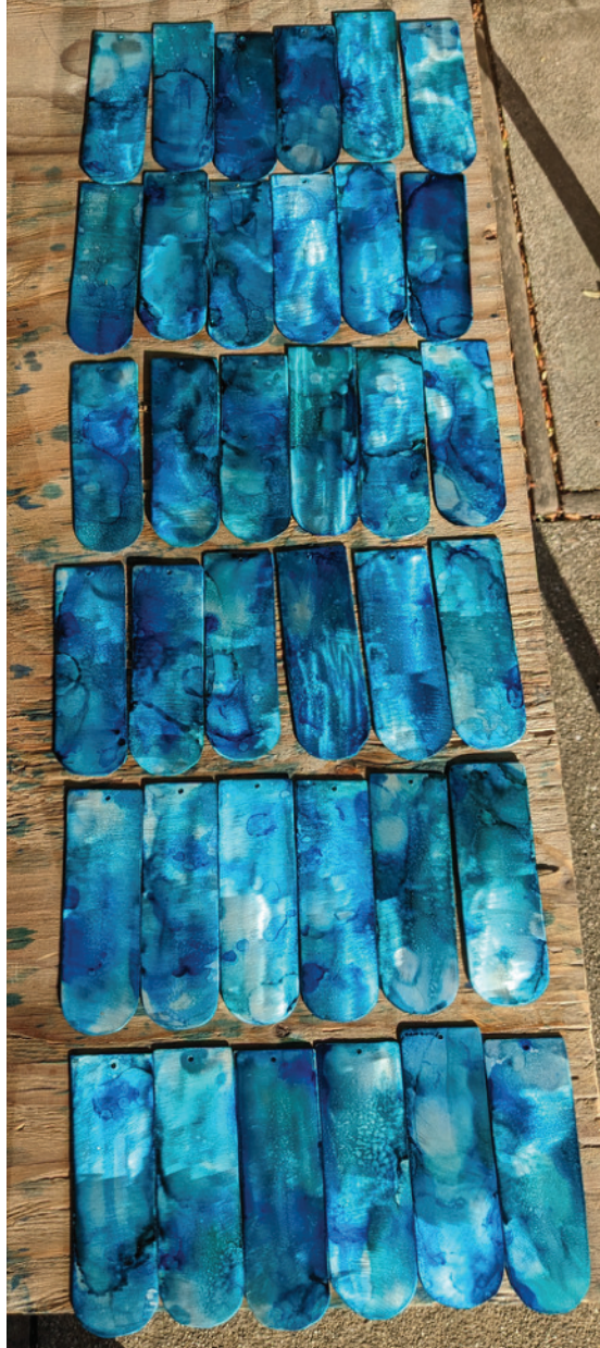
Aluminum Flappers 5052 AL 1/16"x4"x12" Alcohol ink color appli- cation with powder coat clear coat sealant
